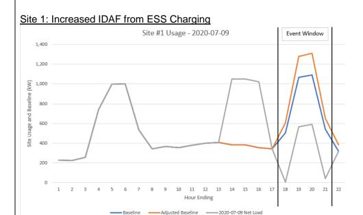
Site #1 shows a theoretical energy storage site charging during the inday adjustment period and then discharging during the event. Despite only providing 500 kW of capacity, the site is credited with an average performance of 660 kW. When this takes place alongside an additional 10 MW aggregation that is responding for 5 MW, the effect is more pronounced. With the site being credited with almost 1200 kW of Capacity.
