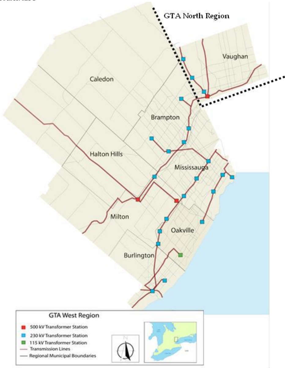
Figure 1 Geographical Area of the GTA WEST Region with Electrical Layout
