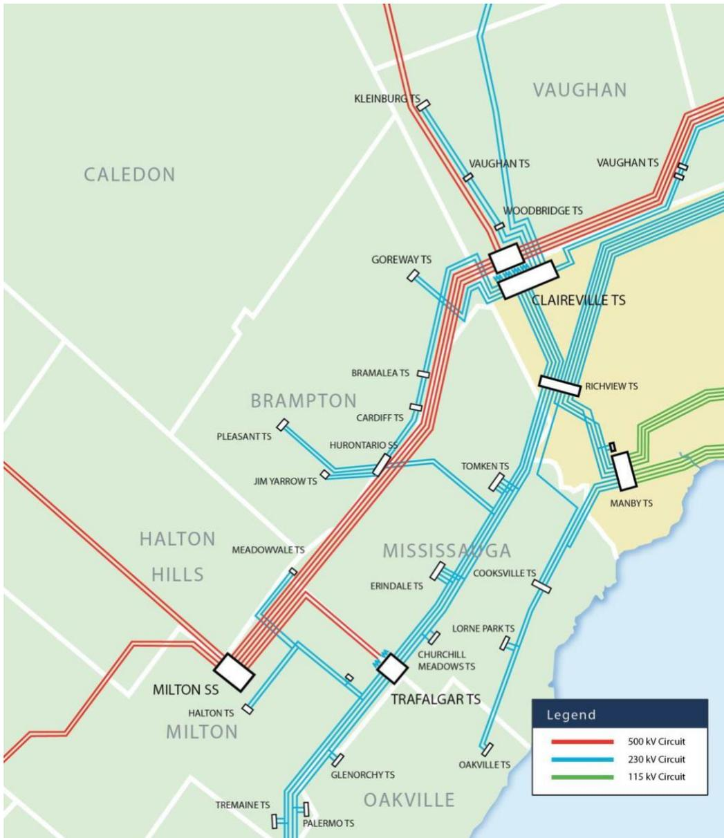
**Figure 2 GTA West Region (Single Line Diagram)**
