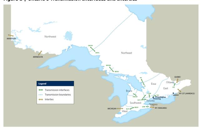
Figure 1 | Ontario's Transmission Interfaces and Interties
