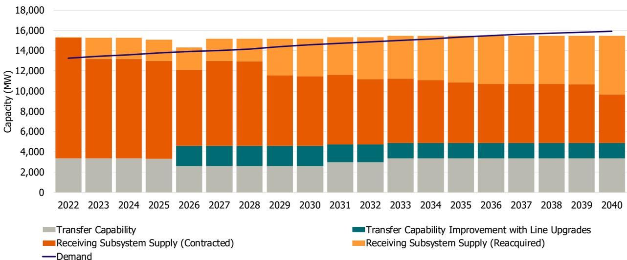
The proposed line upgrade is a flexible solution, in that additional transmission upgrades to further increase transfer capability across FETT can be incorporated in a staged manner at a later date. While not currently anticipated in the near to medium term, the need in the second stage may be triggered depending on future resource acquisitions or other bulk and local transmission needs.
