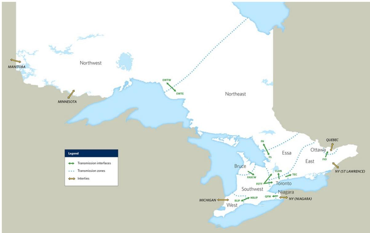
The maximum amount of power that these interfaces and interties can deliver is known as their transfer capability, which reflects constraints to ensure system stability, voltage performance, and acceptable thermal loading.
