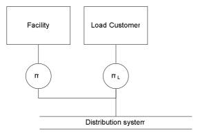
"In Series" means the meter for the Facility is located downstream of the meter for the associated load customer or premises, as follows.
