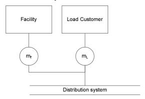
"In Series" means the meter for the Facility is located downstream of the meter for the associated load customer or premises, as follows.
