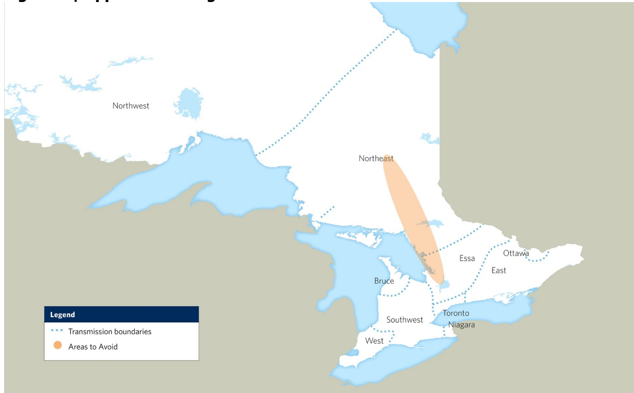
Figure 7 | Approximate Region of Circuits to Avoid Due to Potential IBR Issues
