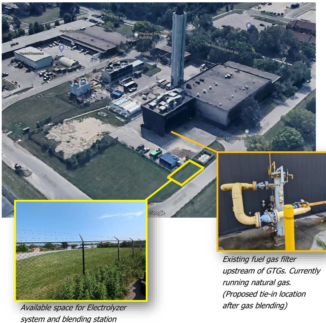
Figure 9 | York University Keele Campus proposed tie-in point and Electrolyzer location
