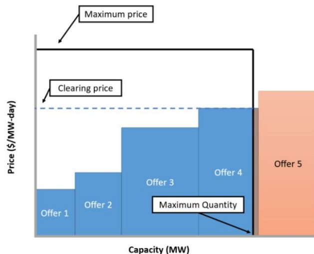
Figure 31 | Process of selecting the DR participant and determining the clearing price based on the IESO/Toronto Hydro required capacity.
