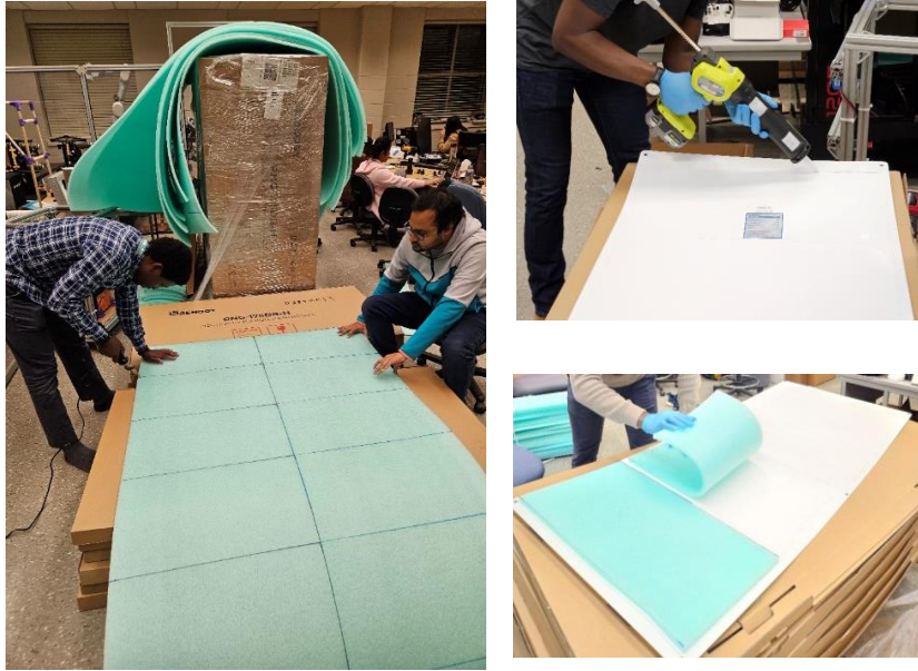
Figure 4.3.18. Assembly procedure of a foam-based floating PV module
