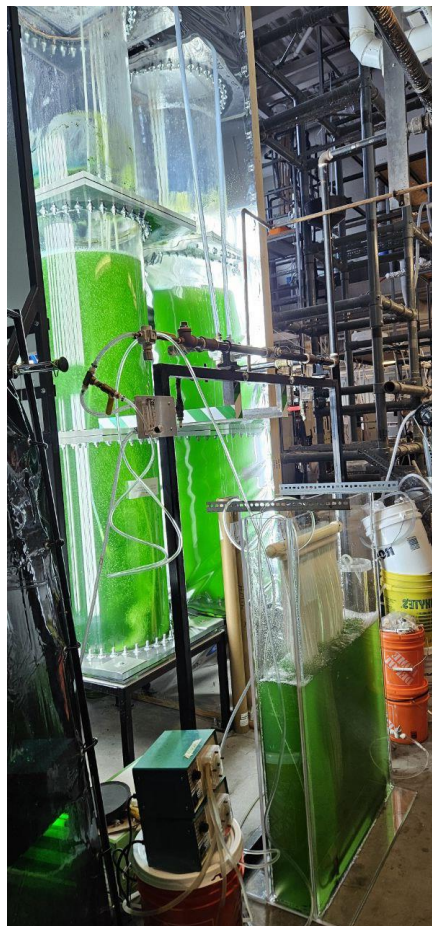
Figure 4.4.4: Photograph of the 500 L bioreactor with the ultrafiltration cell harvesting system
