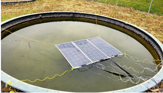
Figure 4.3.17. Installed mini pilot floatovoltaic system at WIRED (In small human-made pond). Design and Installation of 7kW foam-based FPV system
