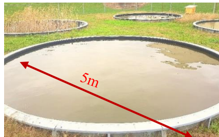
Figure. 4.4.3: Pond photobioreactor for on site microalgal cultivation
