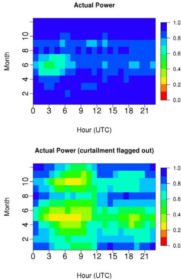
**Figure 2.2: Typical data recovery at an operational plant. The top panel corresponds to the actual power generation, including all plant losses. Bottom panel is actual power generation without curtailment.**
