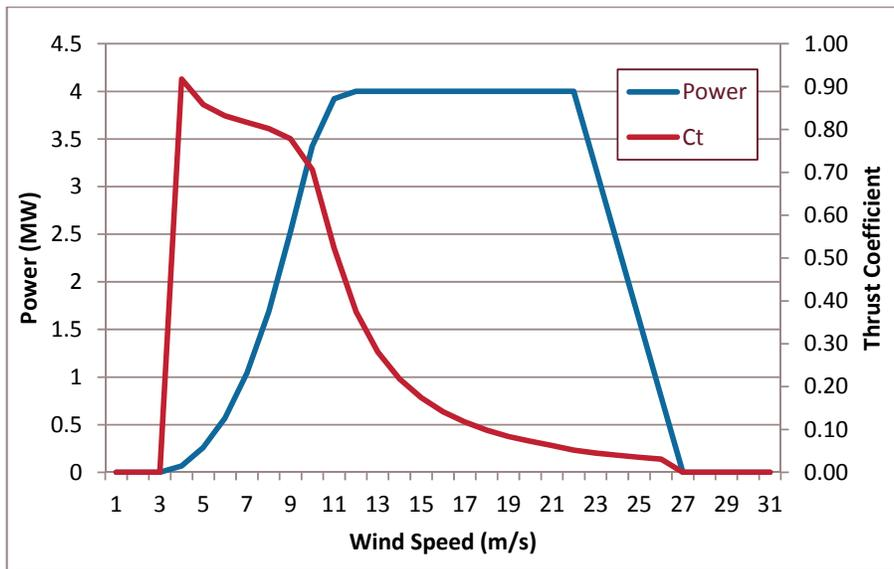
**Figure 3.2: Future technology turbine power and thrust curves**
