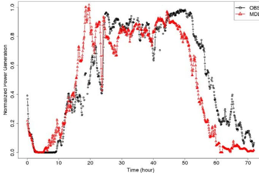
**Figure 5.2: 72-hour sample of 5-minute normalized power generation on February 6 to 8, 2014. The black curve is actual power generation at an operational plant and the red curve corresponds to modeled generation.**
