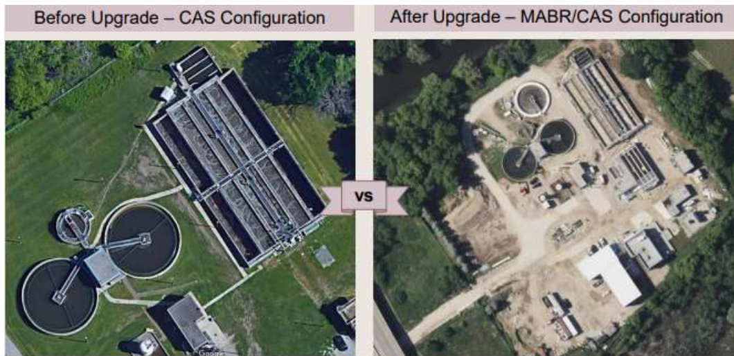
Figure 1: Hespeler WWTP before and after MABR upgrades (Lakshminarasimman & Parker, 2023b)
