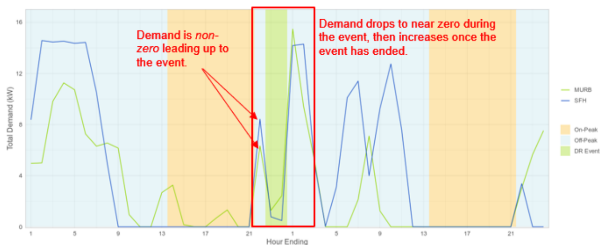
Figure 4 - Total Demand by Building Type, 10 pm to 12 am DR on July 17, 2023. (Source: Generac data, Guidehouse analysis.)
