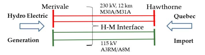
The Hawthorne to Merivale 230 kV Upgrade project consists of reinforcing the existing M30A/M31A circuits between Hawthorne TS and Merivale TS in the Ottawa area
