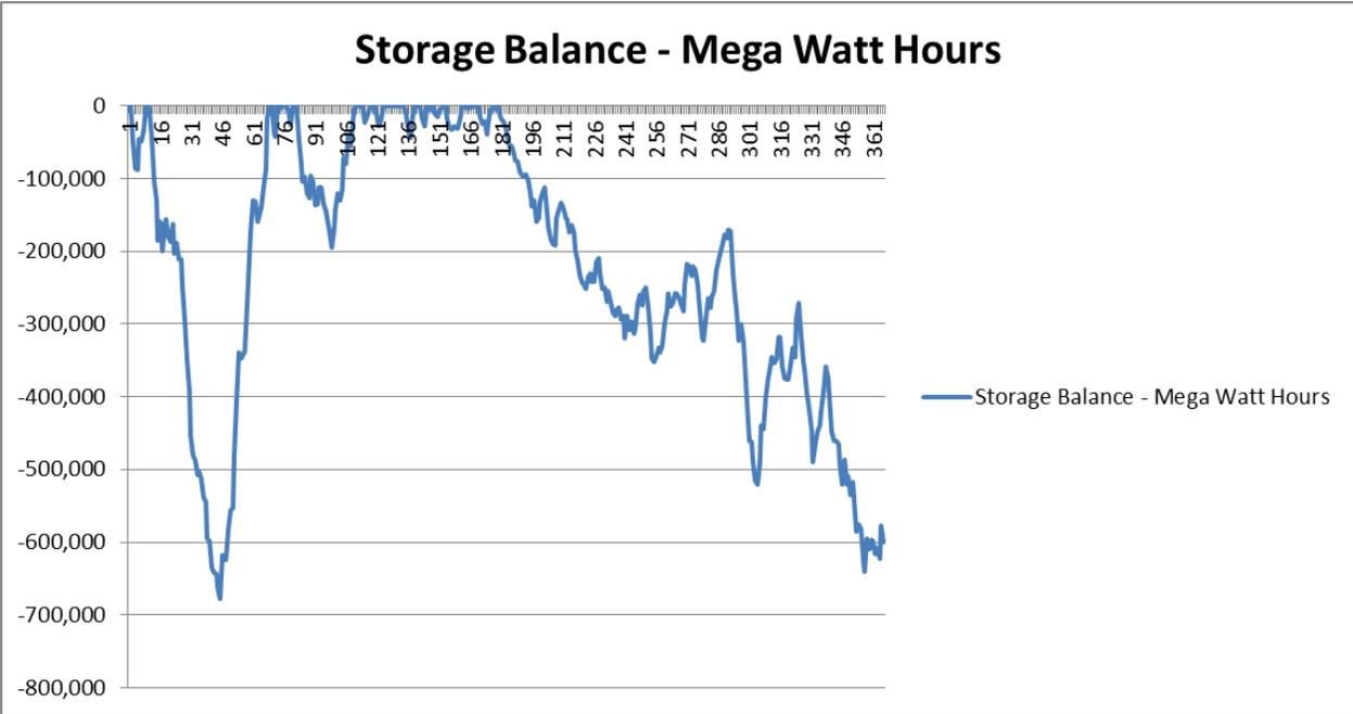
The energy storage requirement in this scenario peaks at about 677 Giga Watt hours. We often hear about storage in conjunction with renewable energy. Generally this is referring to short term storage to facilitate voltage and frequency stabilization on the grid; essentially providing a buffer between the variable power generated and the electrical grid.
