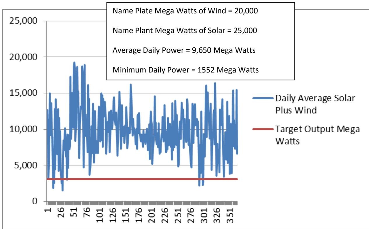
In this run of the model there are only nine days where the daily power output dropped below 3.1 Giga Watts and it never dropped below the 50% threshold. That is the good news. The bad news is that in order to achieve this it was necessary to provision more than three times the target average daily power.
