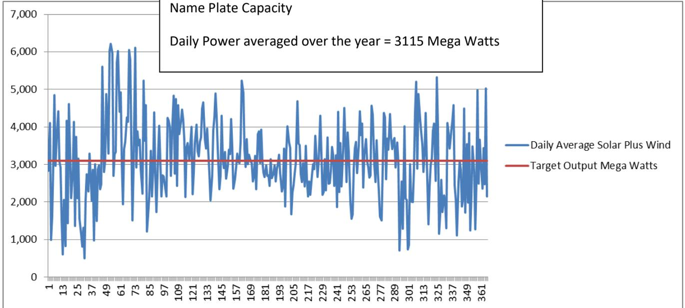
The chart above represents the best attempt to flatten the power over the year. In theory, if we ignore any losses associated with storage we should be able to store the power that is above the target output and then use it when the power falls below the target.
