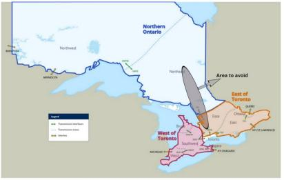
\* The "Area to avoid" in the figure represents the approximate region of circuits to avoid due to potential SSR issues
