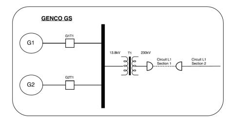
Figure 3-1: Single-Line Diagram Example
