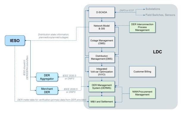
Figure 11: Approach 1 conceptual architecture for LDC operational systems and interfaces
