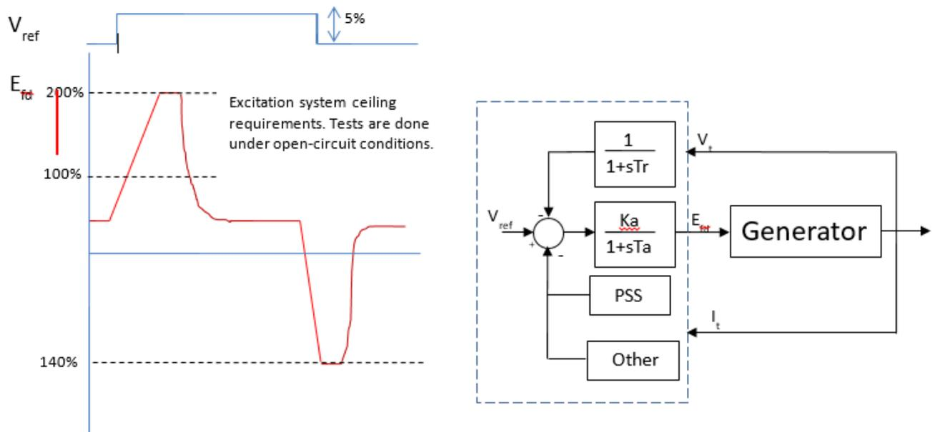
Figure 16 - Excitation System Ceiling Requirements
