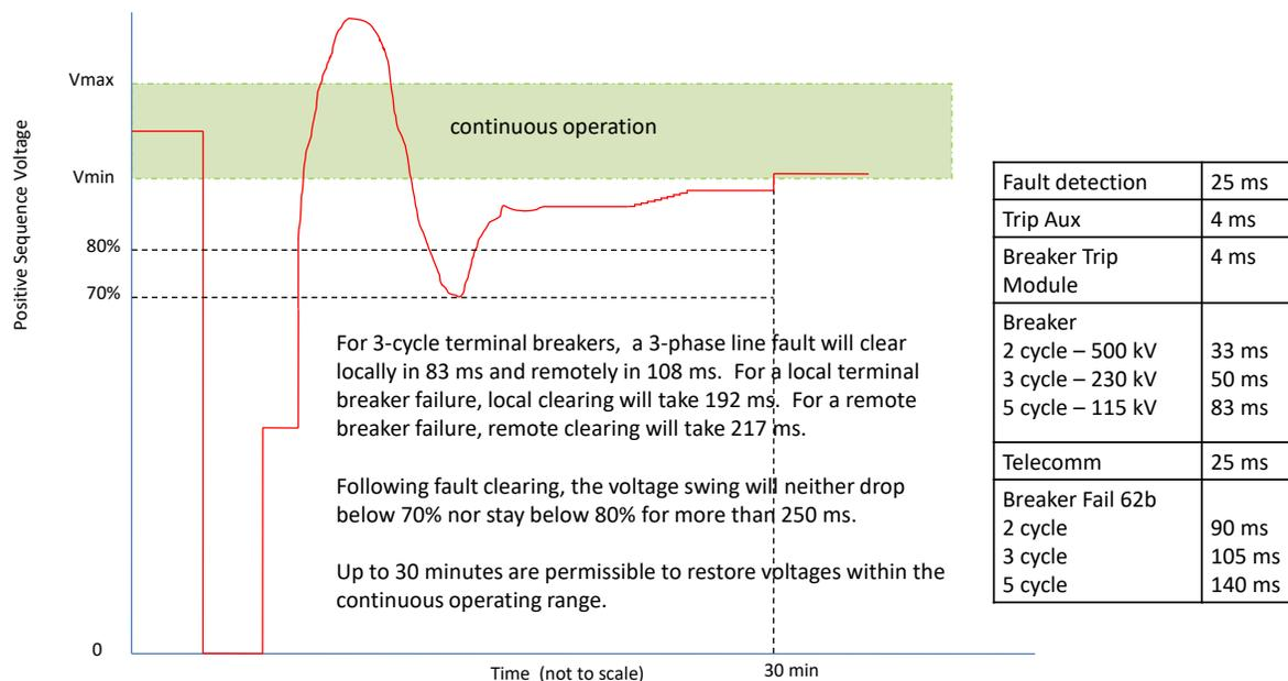
**Figure 9 - Positive Sequence Voltage During a Fault**
