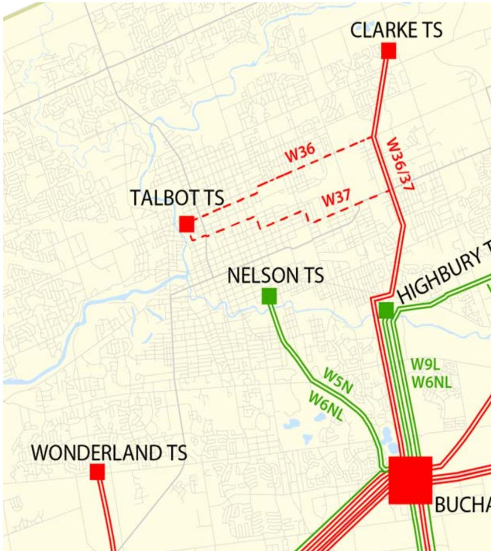
In accordance with ORTAC, all loads in excess of 250 MW must be restored within 30 minutes, and all load in excess of 150 MW within four hours, following the sudden loss of the W36/37 circuits. Given the proximity of emergency crew and equipment, all loads should be able to be restored within eight hours through conventional transmission supply in the Greater London Sub-region.
