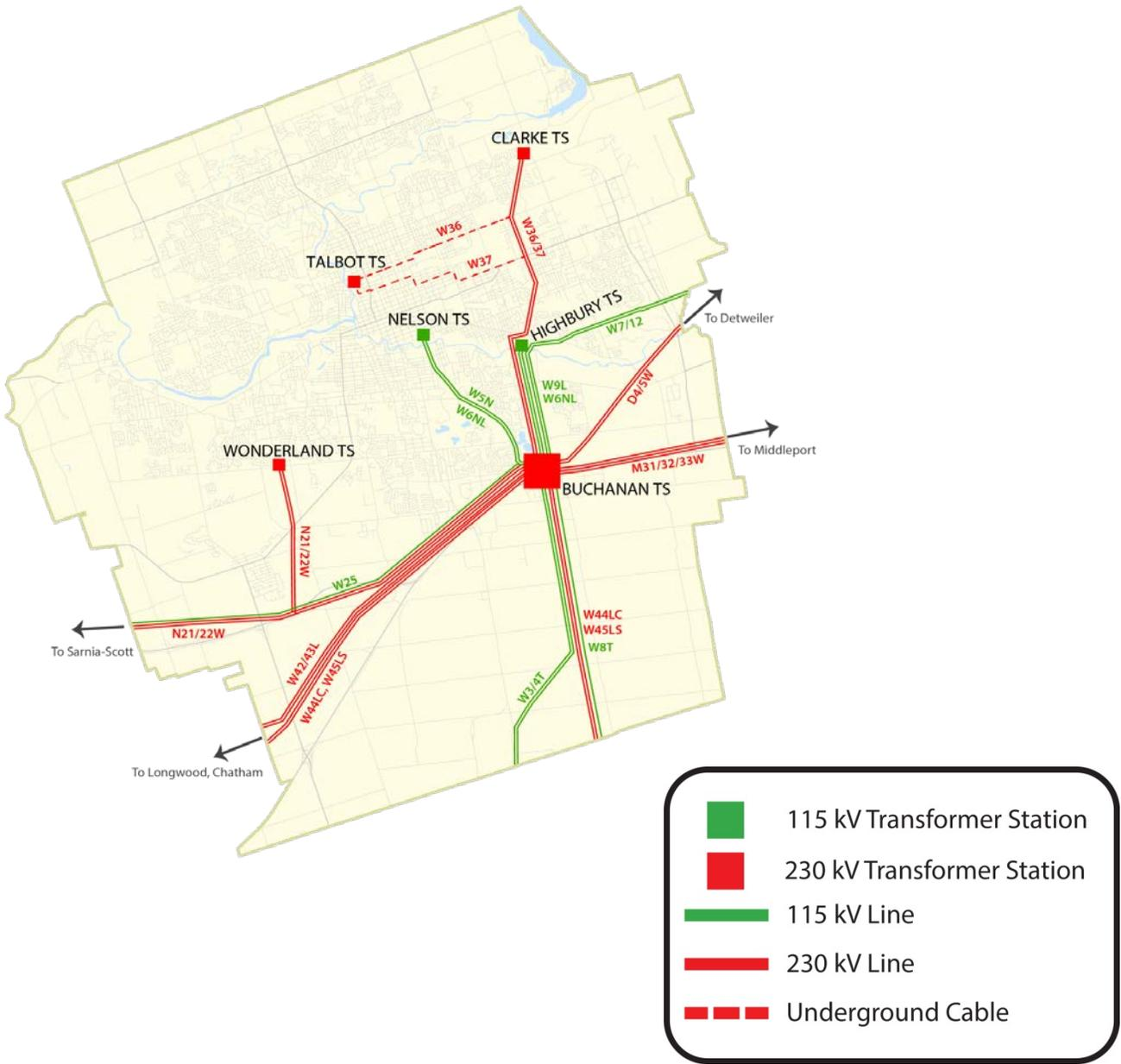
Figure 4-2: Greater London Sub-region Electrical System Configuration
