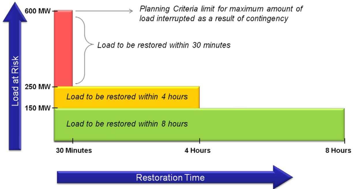
ORTAC indicates that, for the loss of two elements, any load in excess of 250 MW should be restored within 30 minutes and any load in excess of 150 MW should be restored within four hours. The criteria also indicates that any further load below 150 MW to be restored within eight hours
