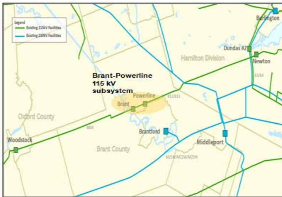
Figure 2-1: Brant Area Electricity System
