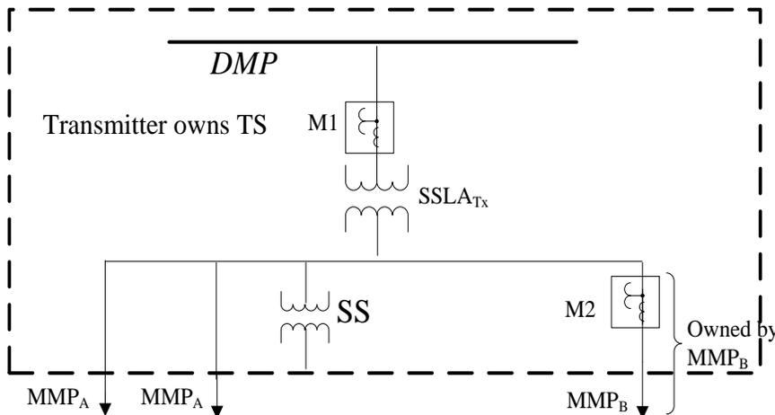
$MMP_A$  and  $MMP_B$  are directly connected to the TS bus inside the fence
