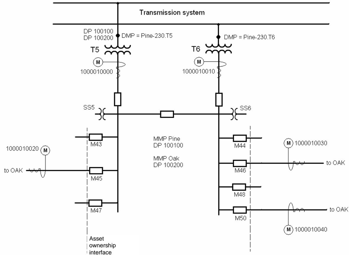
Figure C-1: Single Line Diagram for Pine TS T5/T6
