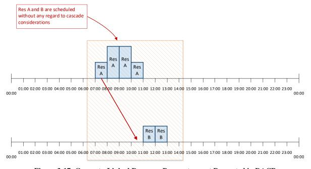
Figure 3-17: Current - Linked Resource Parameters not Respected in DACP
