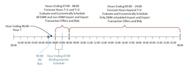
Figure 3-32: Imports and Exports Evaluated for the 05:00 EST PD Calculation Engine Run
