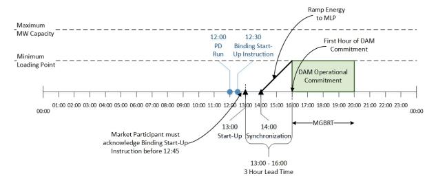
Figure 3-22: Binding Start-Up Instruction (all times in EST)
