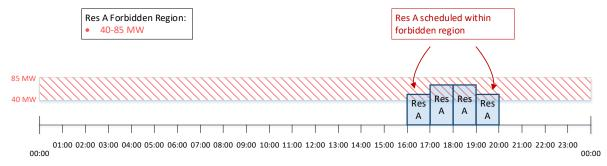
Figure 3-7: Current - Forbidden Region Parameter not Respected in DACP
