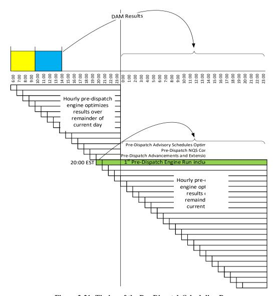
Figure 3-21: Timing of the Pre-Dispatch Scheduling Process
