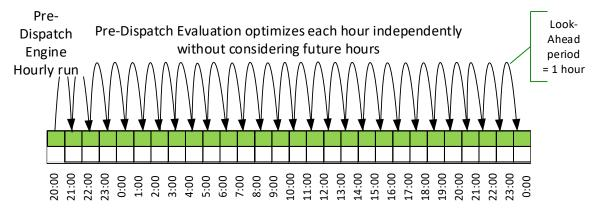
Figure 2-3: Pre-Dispatch Calculation Engine Optimization in the Current Market
