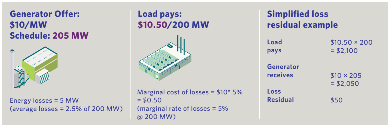
FIGURE 6: EXPLANATION OF LOSS RESIDUALS
