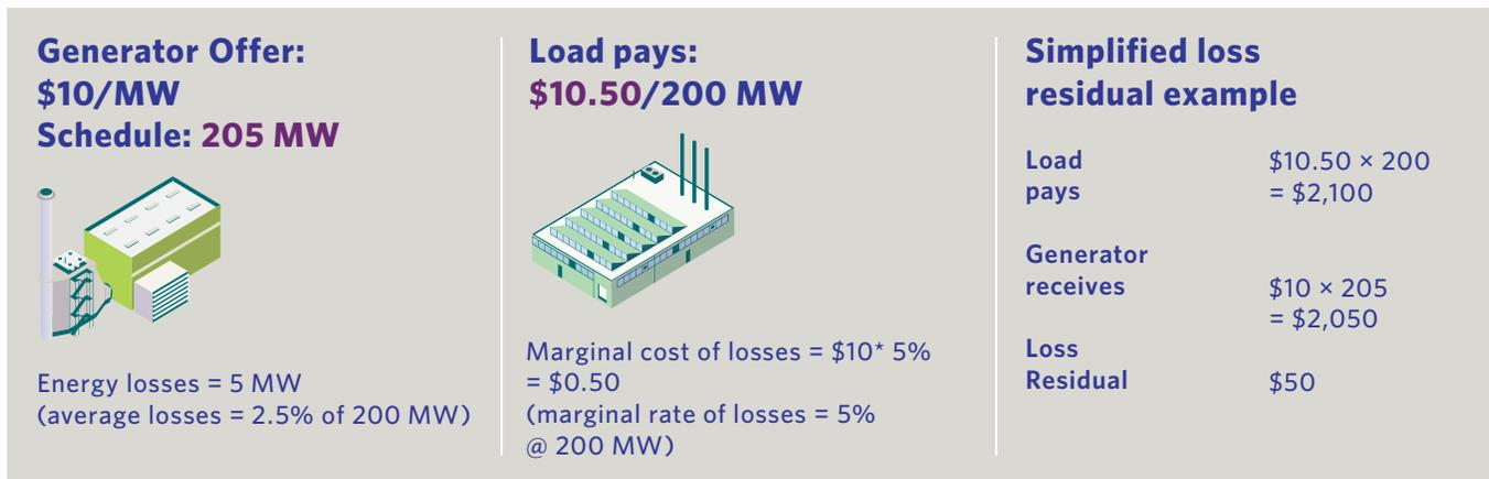
Loss residuals are created even in a simple system with one load and one generator. Due to transmission losses, the generator in this example is dispatched to 205 MW to meet the demand (200 MW) at the load. The price at the load is higher than the price received by the generator.
