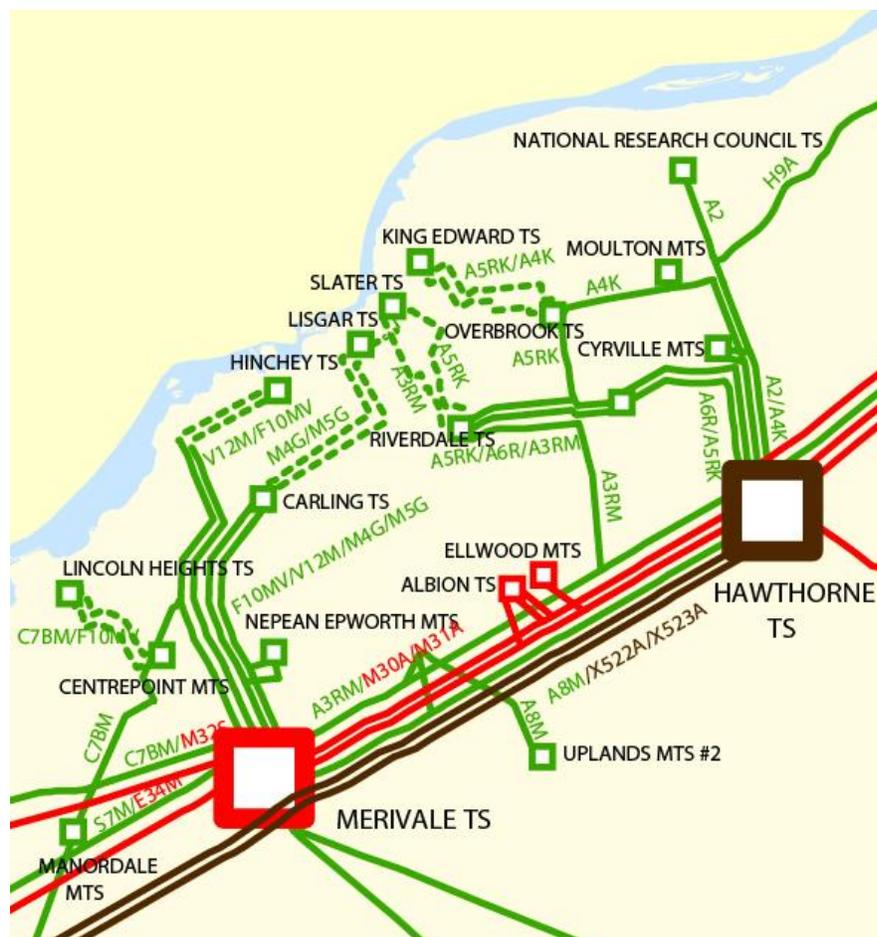
Demand growth on the 115 kV system is increasing the power flow through the 230/115 kV transformers to the point where they are generally reaching their LMC. This issue was identified prior to the 2015 IRRP. At that time, the Working Group determined that sufficient time and mitigating options were available to defer the decision on a plan for the 115 kV system. A plan for long-term reliable supply to the 115 kV system must be confirmed in the near future.
