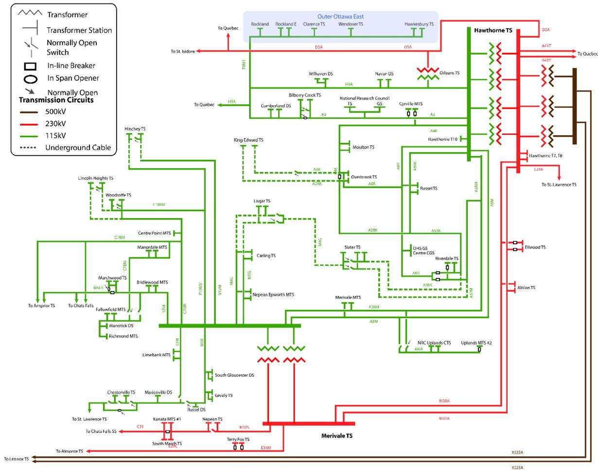
Transmission supply to the sub-region is provided through a 500 kV double-circuit bulk system transmission line connecting to Hawthorne TS, a major TS on the eastern side of the city, and an expansive network of 230 kV and 115 kV transmission lines. Hawthorne TS and a second major TS on the west side of the city, Merivale TS, are the two main supply points for the sub-region. These stations have a total of six 230/115 kV transformers providing supply to the 115 kV
