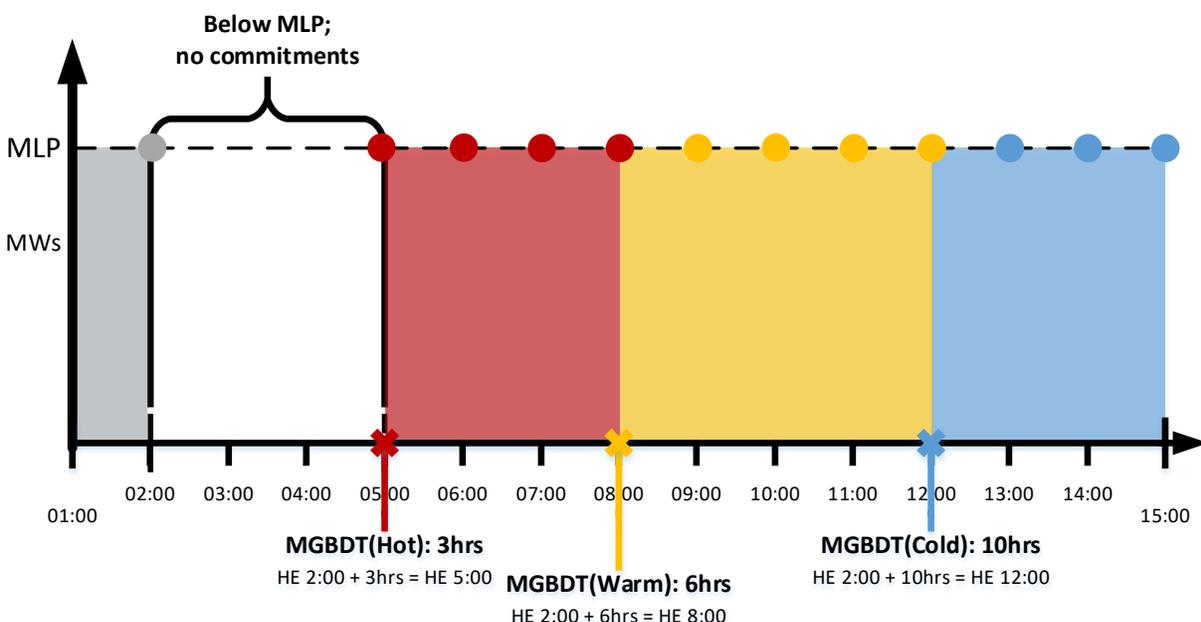
In the example in **Figure 6**, Generator A is dispatched below its MLP at 02:00. Based on its MGBDT data (i.e. hot MGBDT of 3hrs), it cannot be scheduled to reach MLP again until at least 05:00. Generator A can
