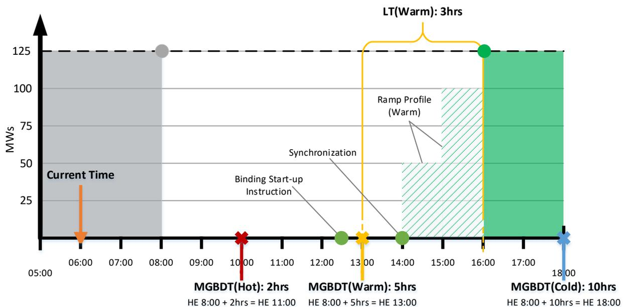
As illustrated in **Figure 7**, the PD scheduling process calculates that there are eight hours between when Generator A will end its commitment at 08:00 and when it will be needed again at 16:00. The scheduling process then determines that Generator A will be warm at 16:00 by comparing the length of the time it will have been below its MLP (i.e. eight hours) to its MGBDT data. Generator A enters a warm state after
