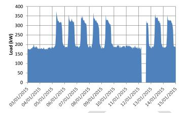
An analysis on other days over similar hours that the load over which the gap appears is not constant, but is repeatable.
