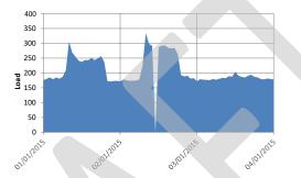
The load just prior to the gap (10:00 AM) was 291 kW and the load just after the gap (12:00 PM) was 287 kW.
