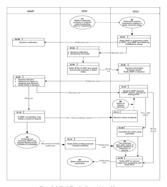
Figure 2-3: Work Flow for Quarantining a Meter
