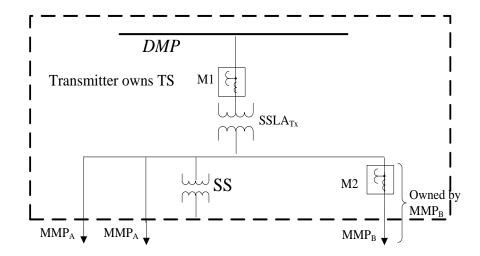
$MMP_A$  and  $MMP_B$  are directly connected to the TS bus inside the fence  $MMP_A$  and  $MMP_B$  are  $\it transmission \it customers$
