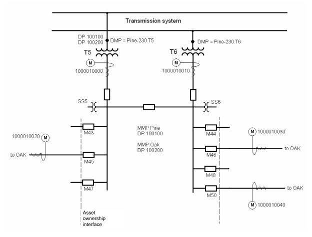
Figure C-1: Single Line Diagram for Pine TS T5/T6
